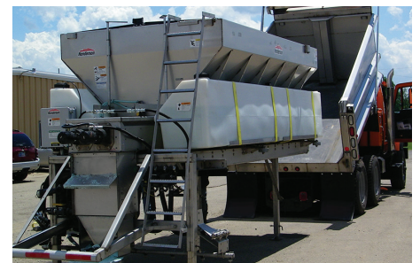
OPTIONAL: Air flow baffle mounted ahead of the liquid spray boom helps prevent drift due to travel speed and wind turbulence.
