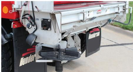
Spinner assembly is self-leveling regardless of dump body angle, without the need for a stabilizer bar. It is adjustable both vertically and horizontally. Vertical adjustment allows for fit to different chassis/dump body sizes, while the horizontal adjustment allows for changes in spread pattern.
