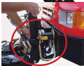
STEP 2 Raise protective cover of the quick-connect fittings. Depress red button, then raise the lever to upright position.
