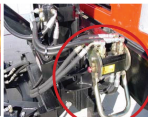
Insert hydraulic connection block, pivot handle and you are connected! No oil mess-even under pressure!
