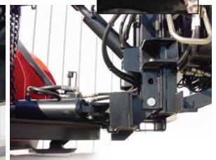
STEP 4 Raise jack (using bumper-mounted switch) to secure both halves of the plow hitch together. Install safety pin, connect plow lights and you are ready to roll.
