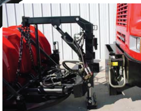
STEP 1 Drive up and align truck portion of hitch with the plow portion of hitch.
