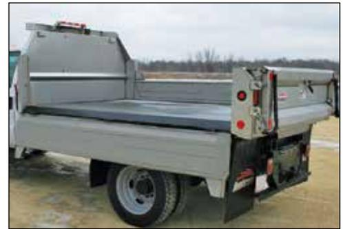
**OPTIONAL** contoured, tapered headsheet is aerodynamically shaped to complement the new cab designs and increase visibility.
